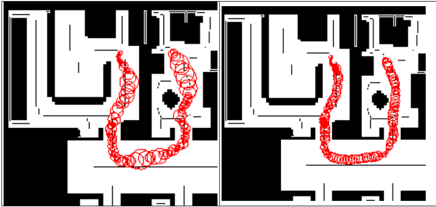
Fig. 1. Two behavior traces produced by the same navigation plan and local navigation module using different plan execution mechanisms. The robot's position is depicted by a circle where the size of the circle is proportional to the robot's translational speed.
